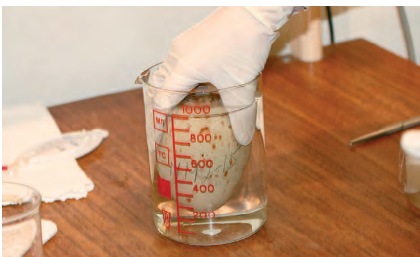
The so-called float, i.e., measuring the fertilization of eggs. Photo: Petr Suvorov
